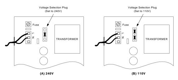
Figure 2.4: Voltage Selection (240V or 110V)
